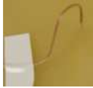
Figure 9 Thermocouple held in place using electrical tape prior to applying epoxy
