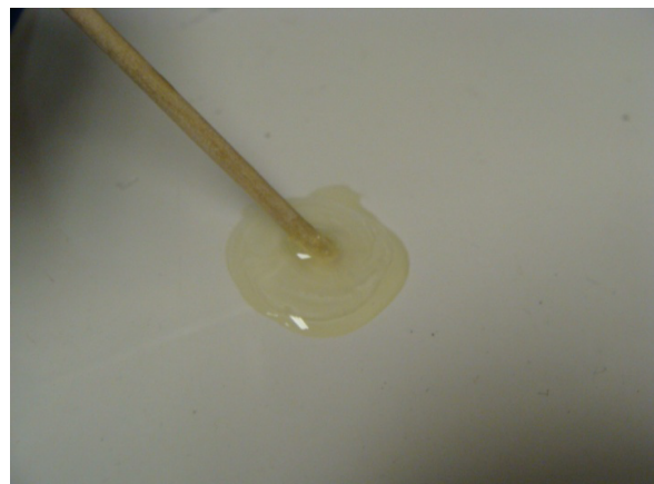
Figure 8 Be sure the epoxy is well mixed
