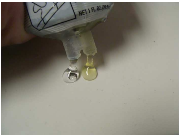
Figure 7 Dispense 2-part epoxy on clean surface
