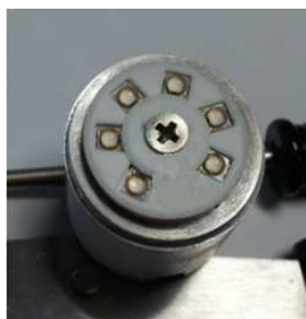
Figure 24 Flat head screw recommended
