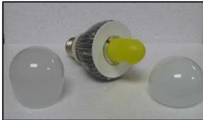
Figure 19 Large globe (left), test bulb (center), small globe (right)
