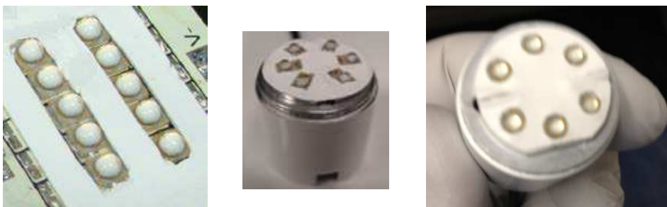
Figure 23 Mixing chamber material around LED arrays
