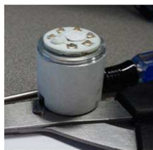
Figure 25 Reflective material on screw = 5% gain
